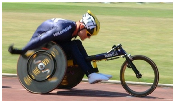
Figure 5 - Bob Hall's three wheeled chair design for sprinting (Mandeville Legacy, 2014)
